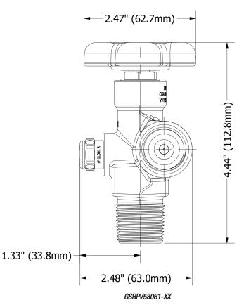
Residual pressure valve designed to protect cylinder and contents.
