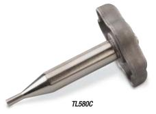
Gas cylinders can be checked for content integrity by simply inserting the Checking Rod and pushing against the resistance of the check valve. The sound of escaping gas indicates residual cylinder pressure.
